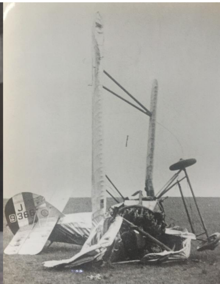
Siskin IIIa crashed by Flight Cadet Clarkson. Landing with drift caused this type of prang - which was fairly common! Known in those days as a 'Chinese Three Pointer' - one wheel, one wing and the tail skid.
