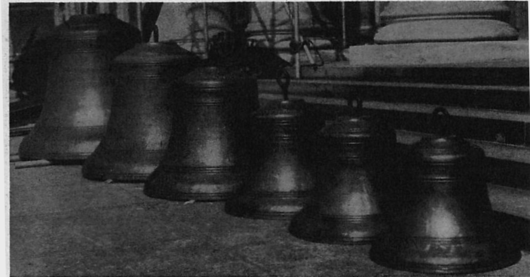
The Bells before installation in the Tower. Here all six bells lie at the foot of the steps leading up to the main entrance of the College. The notes and sizes of the bells are: G (2 cwt.), F (2½ cwt.), E flat (3½ cwt.), B flat (7 cwt.), G (13 cwt.), E flat (25 cwt.). The four smaller bells are used for the Westminster Chime, the four larger ones for sounding 'Retreat.'
