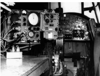
H2S equipment on the left
